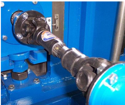
Notice the spline in the middle of this driveshaft connecting the two components and transferring torque.
